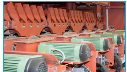
Abb. 11: Sägeaggregate
