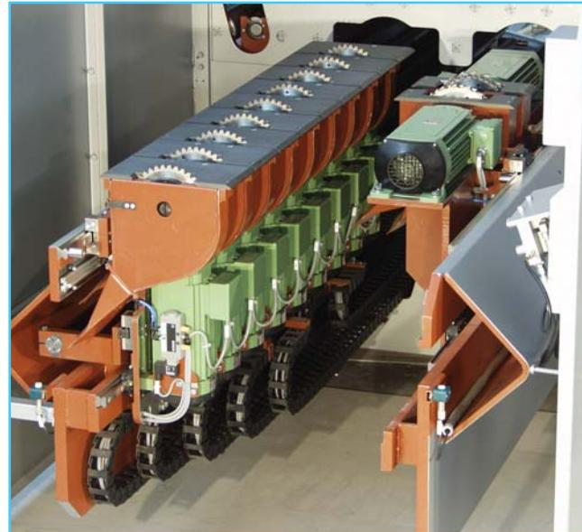
Abb. 6: Sägeaggregate in Parkposition.
